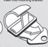
STEP 4: Fold back strap again and insert through bottom portion of buckle.
